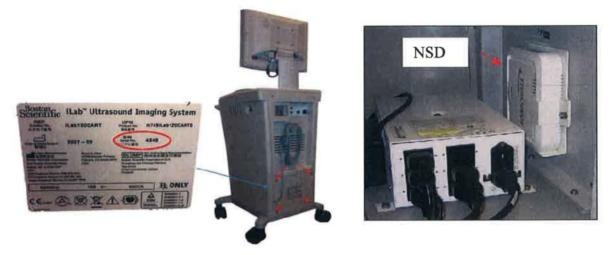
Integrated Systems – The serial number is found on the on the top of the isolation transformer. In typical installations the isolation transformer as well as the NSD are located in the control room.
